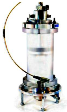
Cellule insertion pieux \sigma_3 \text{ max} = 200 \text{ kPa} Echantillon: \Phi = 70\text{mm} h = 100\text{mm}
