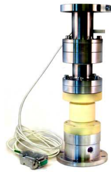
Nano-cellule TX roches \sigma_3 \text{ max} = 20,000 \text{ kPa} Echantillon: \Phi = 1\text{mm} h = 2\text{mm}
