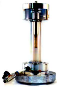
Cellule triaxiale granulaire \sigma_3 \text{ max} = 1000 \text{ kPa} \sigma_1 \text{ max} = \sim 7000 \text{ kPa} Echantillon: \Phi = 11\text{mm} h = 22\text{mm}
