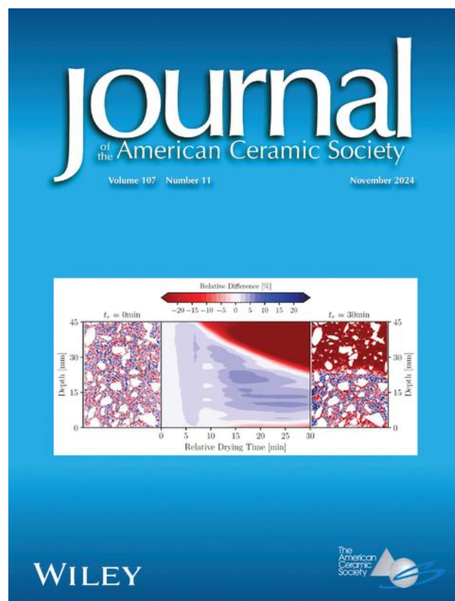
Figure: Cover Photograph: Residual moisture in refractory castables can lead to explosive spalling. Understanding water transport mechanisms is key to improving the longevity of these critical manufacturing tools. In-situ visualization using neutron tomography shows both drying fronts (dark red) and internal water accumulation (dark blue) for a castable containing cellulose fibers.
