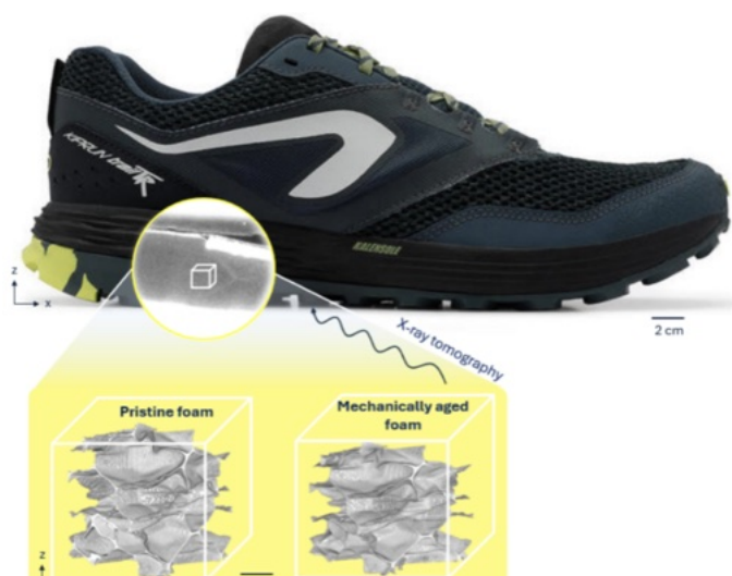
Figure: trail running shoe with a zoom on the 3D cellular structure of its midsole before (left) and after (right) running a 150km trail.
