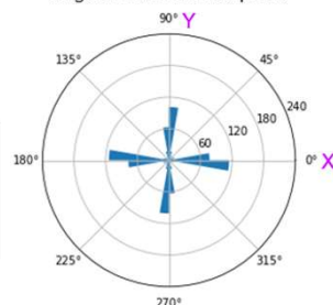
2.a) Orientations of local contacts between grains and the lower geogrid
